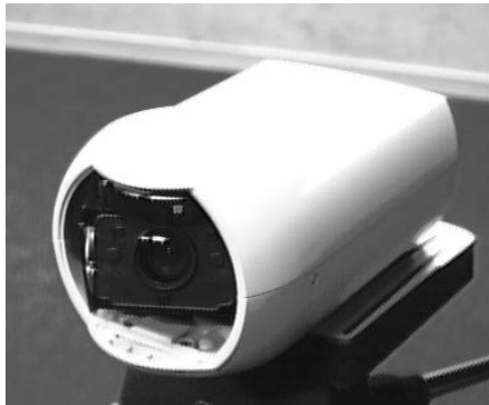
Figure 2.24: Off-the-shelf FV-PTZ camera: SONY EVI-G20.
