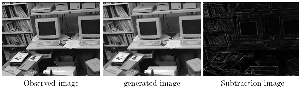
Figure 2.32: Comparison between the observed image and the generated image (Generated image: zoom = 4096, View direction = (-20.0^\circ, 4.0^\circ) ).
