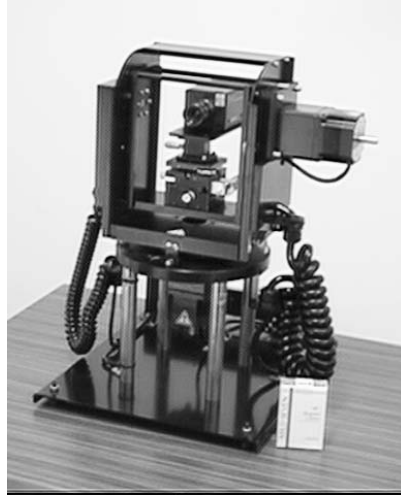
Figure 2.16: Developed FV-PT camera head.
