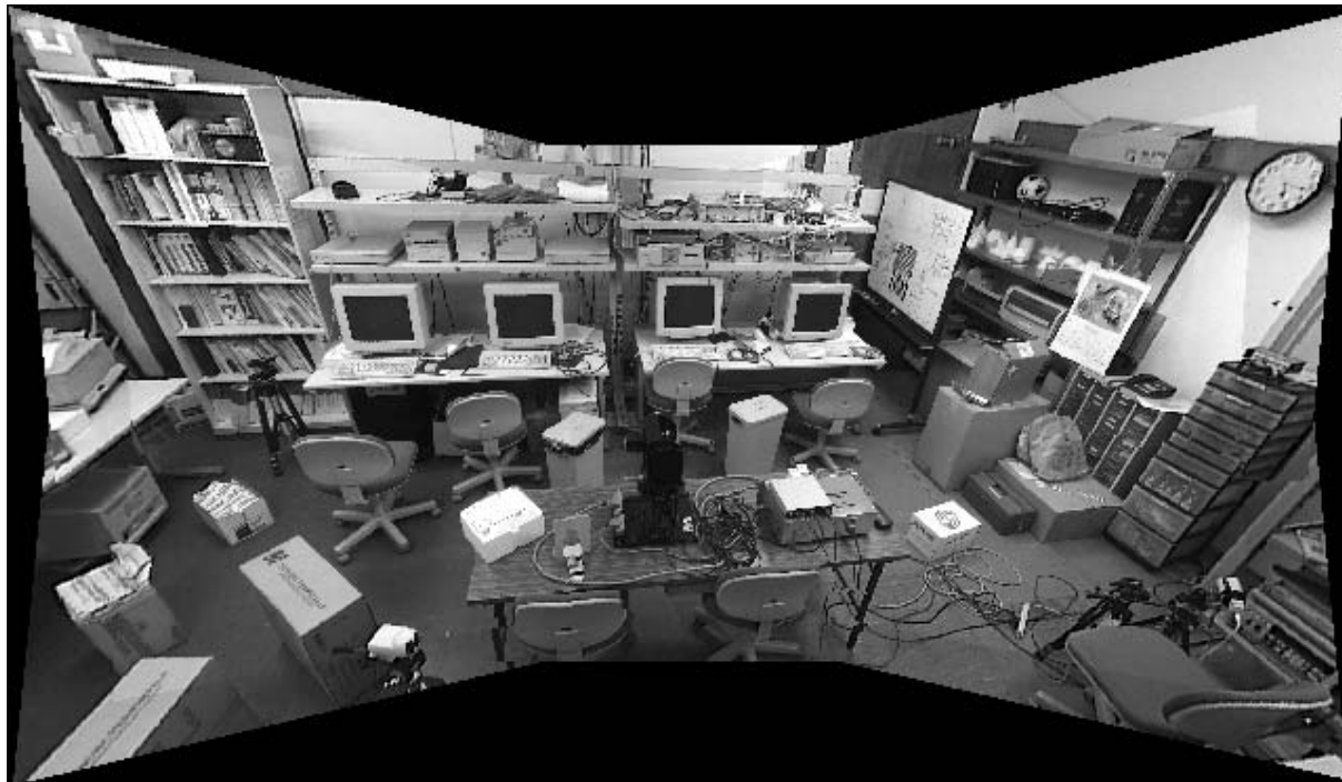
Figure 2.31: High resolution APP ( \rho = 2500.622 [pixel], image size = 6332 \times 3684 [pixel]): the images taken with various zoom parameters are re-projected onto an APP.
