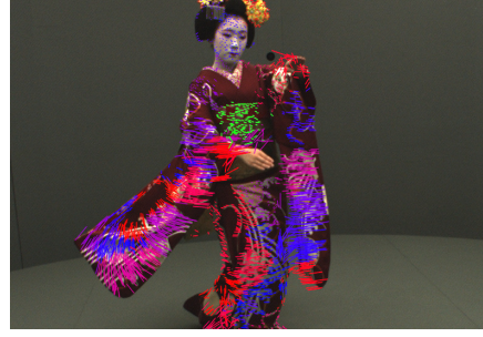
Figure 3. Motion flow clusters. Here, 2941 motion features were detected and grouped in 30 clusters. Spectral clustering is used to cluster optical flows according to length, orientation and position. Piecewise rigidity can be assumed between consecutive frames due to the video frame rate (25fps).
