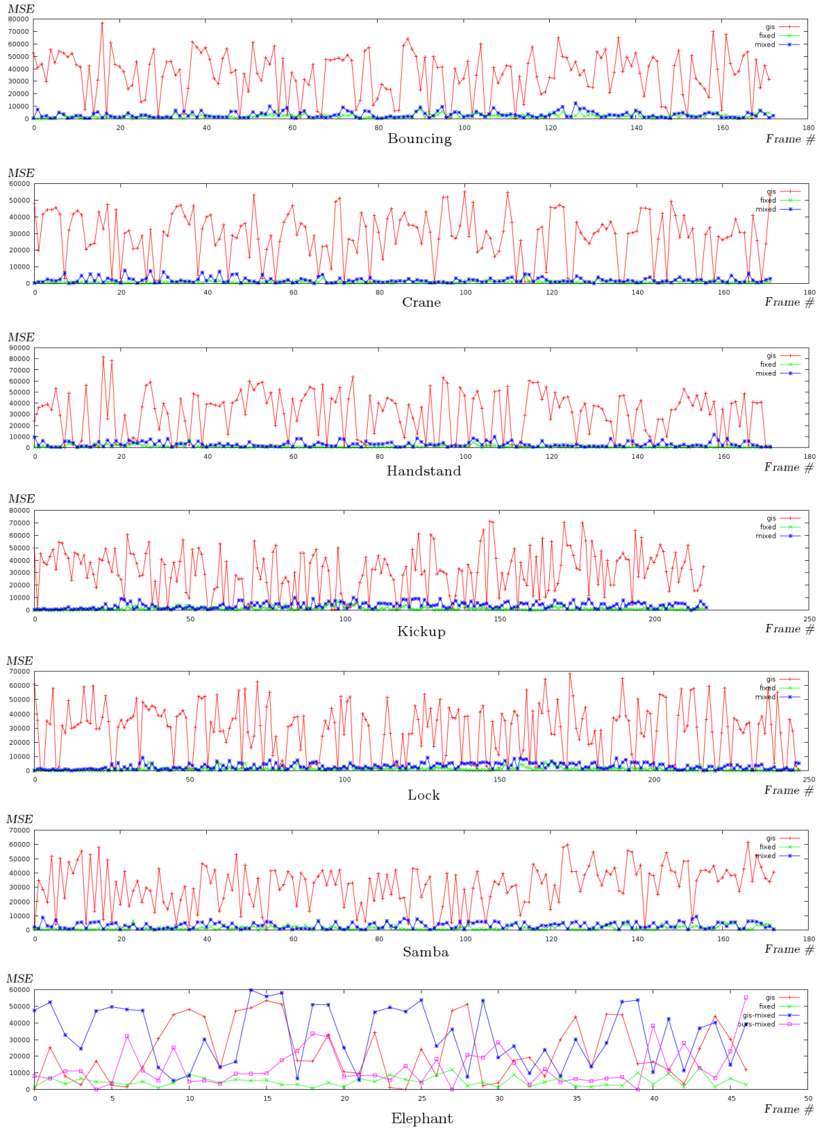
Fig. 9 Mean Square Errors (MSE) of pixels between consecutive geometry images. Results obtained with [39] are denoted 'gis', results obtained with our method on sequences with fixed resolution are denoted 'fixed', and results obtained with our method on sequences with mixed resolutions are denoted 'mixed'.
