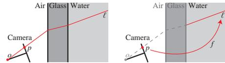
**Fig. 2** Appearance-based calibration. The relationship between a pixel  $p$  and the ray  $\ell$  which passes through  $p$  and the camera center  $o$  (left) is modeled by a function  $f : p \rightarrow \ell$  without knowing the geometry of the refractive layers (right).
