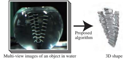
**Fig. 1** 3D shape reconstruction of objects in water from multi-view images with refractive distortions. Left: a tripod (upside down) in a fishbowl. Right: reconstructed 3D shape.
