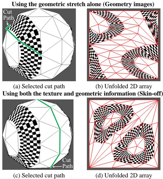
**Fig. 11.** Results of the cut path selection and the mapping onto a 2D array
