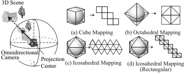
**Fig. 4.** Polyhedral mappings for representing omni-directional video data on a 2D plane
