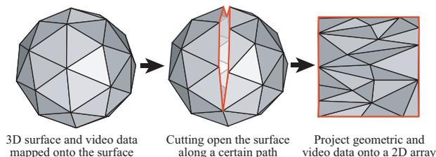
Fig. 1. "Skin-off" operation for representing 3D video data by a 2D array
