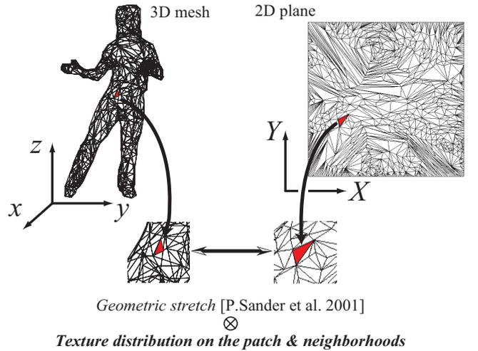
**Fig. 5.** Optimization of mapping function from a 3D mesh to a 2D plane
