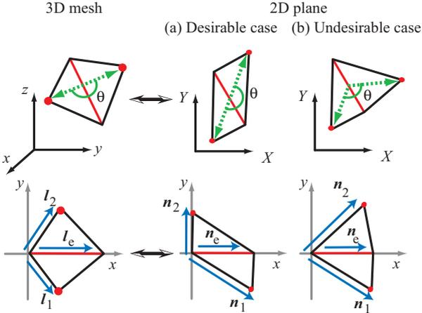
Fig. 6. Stretch direction continuity between adjacent patches
