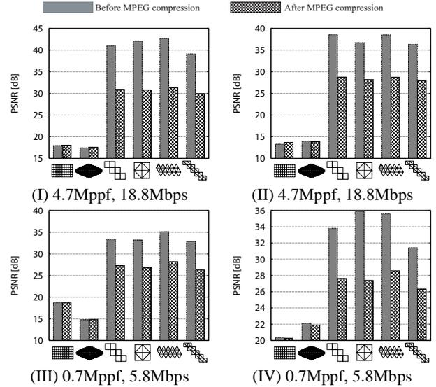
**Fig. 9.** Compression efficiency for omni-directional video
